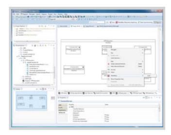
It is realized as an extension of the Eclipse Team Provider interface. The workflow is very similar to the one that developers are used to when working with Eclipse Subversion clients for example. The adapter provides several different views, which show the content of the ModelBus® Repository or the Model-Bus® Notifications for example. The adapter also tracks dependencies of a model to other models including meta-models or profiles. In that way they can be synchronized automatically.
