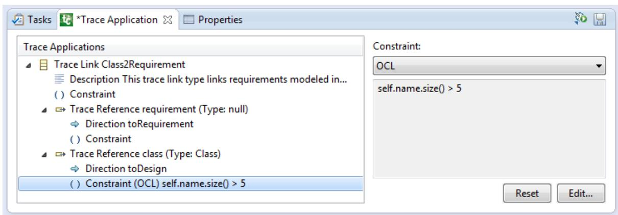
**Figure 17 Specifying a Constraint for a Trace Reference**
