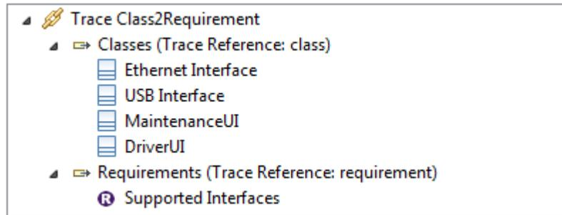
**Figure 27 Hierarchical Representation of a Tracability Link**
