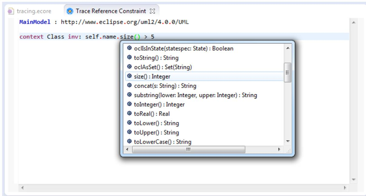
**Figure 18 Topcased OCL Editor Showing a OCL Constraint**
