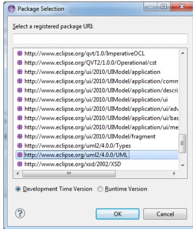
**Figure 11 Loading the required UML meta model package into the EMF Editor**
